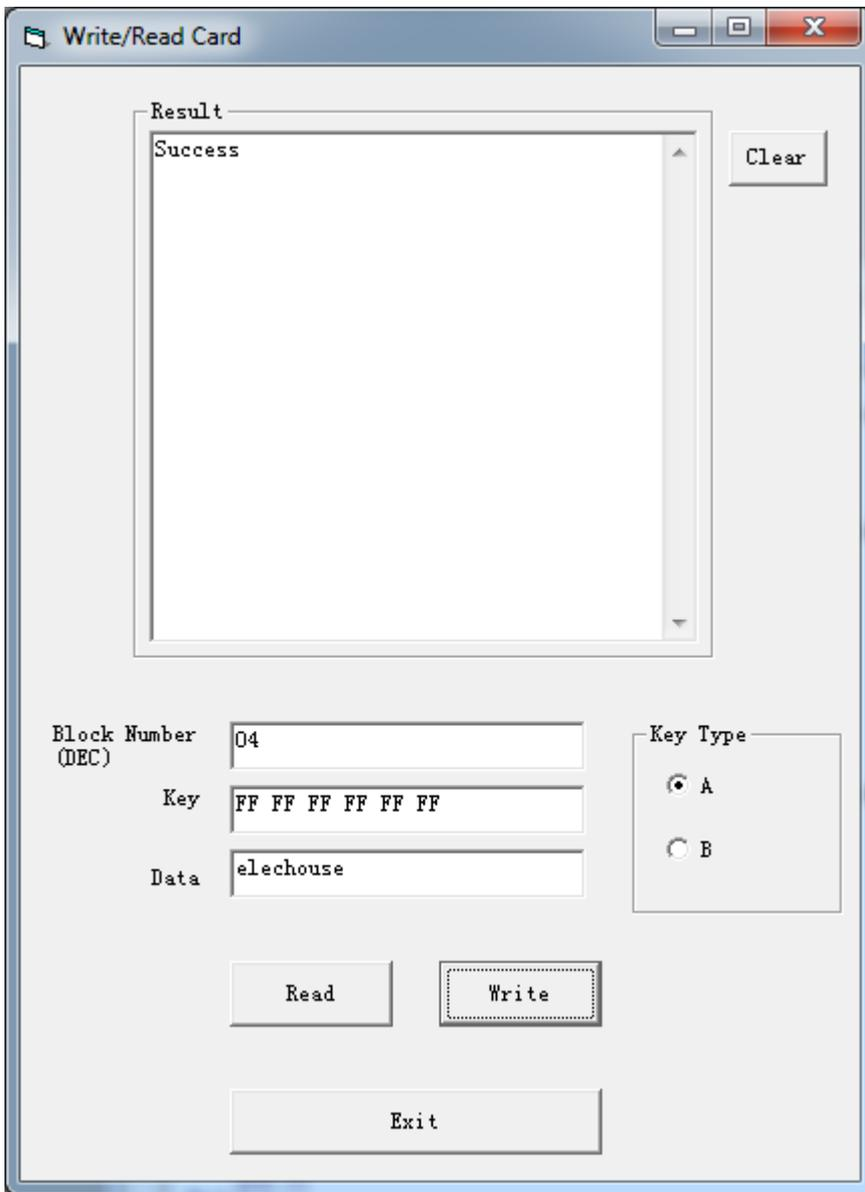
*I will right "elechouse" to the 5<sup>th</sup> data block of IC card (00 is the 1<sup>st</sup> one). Note: not every block could be written.*
